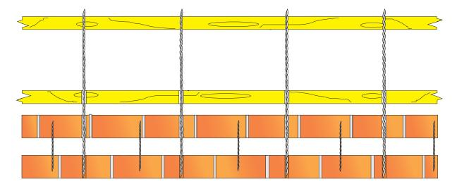
Use Bow-Fix detail BF-02 to tie joists which run parallel to walls install remedial wall tie between Bow-fix ties.
