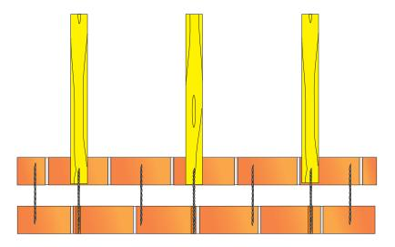
Use Bow-Fix detail BF-01 to tie joist ends which run perpendicular to walls and install remedial wall ties between joists
