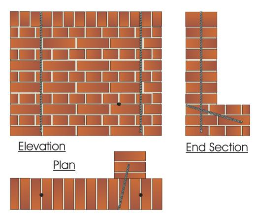
(1) After locating and marking positions of holes on top of wall. Drill a clearance holes (13mm-16mm diameter depending upon material and the length of tie to be used) to required depth.
