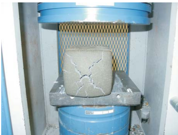
Testing Compression strength
