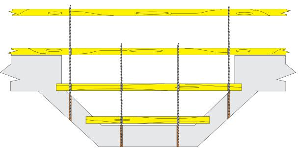
Use Bow-Fix detail BF-02 to tie joists which run parallel to front elevation of Bays
