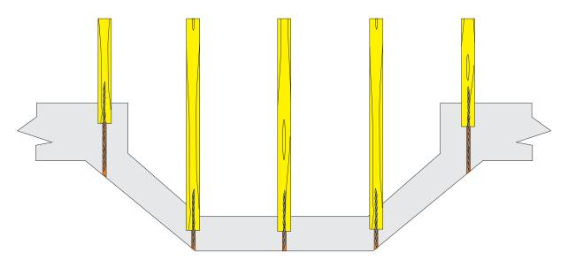
Use Bow-Fix detail BF-01 to tie joist ends which run perpendicular to front elevation of Bays
